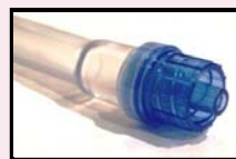
Figure 3. Disposable irrigation tubing’s one-way valve. Displayed is an example of a one-way (primary) “backflow” valve that is embedded into one of this disposable irrigation tubing’s two ends. An endoscope connector attaches to this end, connecting the tubing to the GI endoscope. This valve is intended to prevent both the tubing’s contamination and water siphoning.
