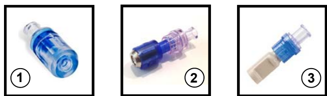
Figure 4. Endoscope (port) connectors. The endoscope connectors marketed by three different manufacturers are displayed. Each of these connectors is intended for single-use and is manufactured with a one-way (secondary) valve, which is primarily designed to prevent contamination of the disposable tubing and its own embedded (primary) one-way valve during GI endoscopy. Manufacturers of disposable irrigation tubing may also market reusable (i.e., "24-hour use") endoscope connectors that are generally designed without a one-way valve, but to which can be attached a separately purchased, single-use one-way valve. 8,9 No matter whether single-use or reusable, the endoscope connector connects the disposable tubing (see: Figure 1 ), to a port that feeds directly into the GI endoscope's auxiliary water channel. In general, these endoscope connectors are accessories that are purchased separately from the tubing. (These images were printed with the permission of their respective manufacturer.)
